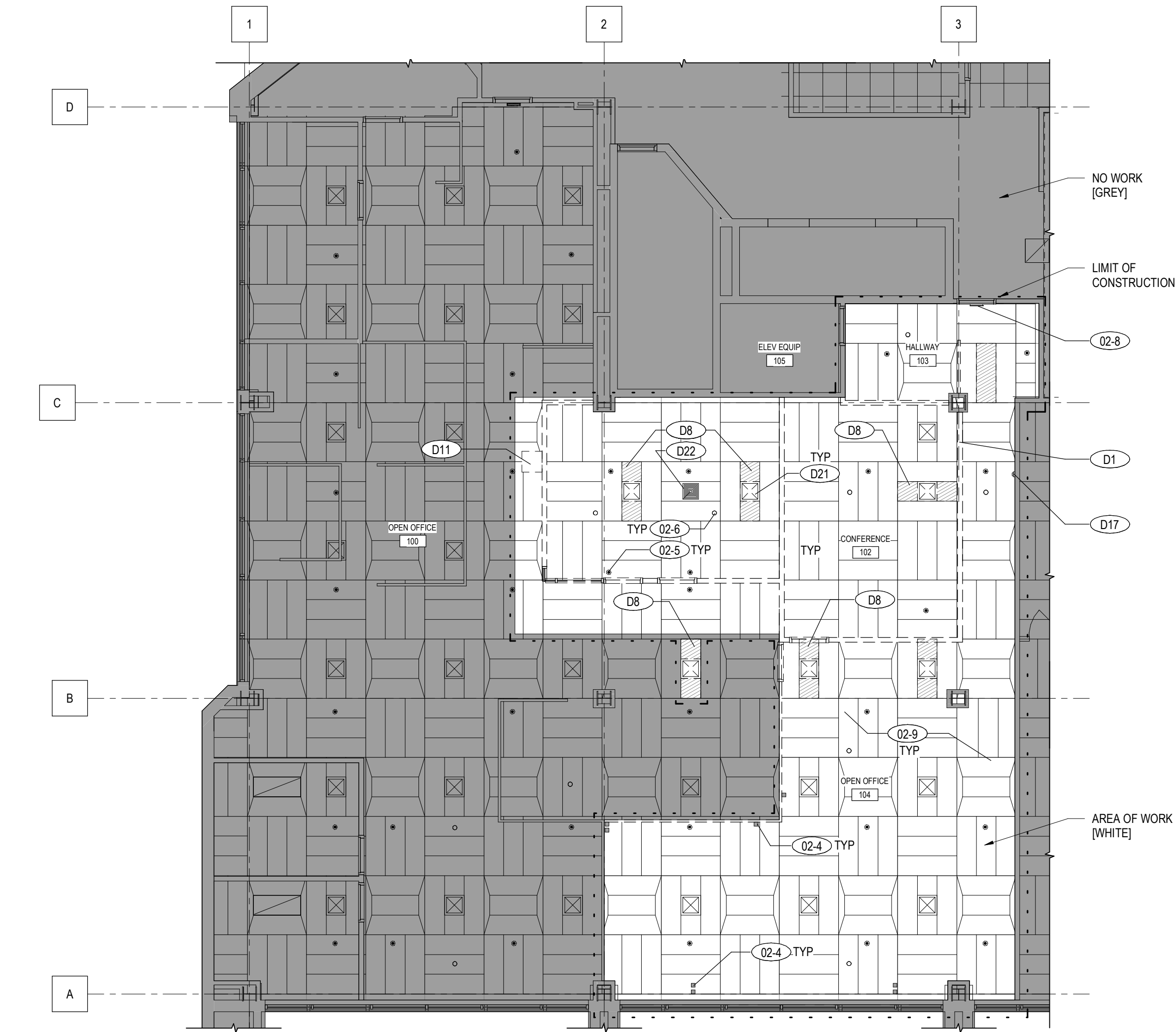
FIRST FLOOR REFLECTED CEILING PLAN - AREA OF WORK - DEMOLITION NORTH 3 AD1 1/8" = 1'-0"
