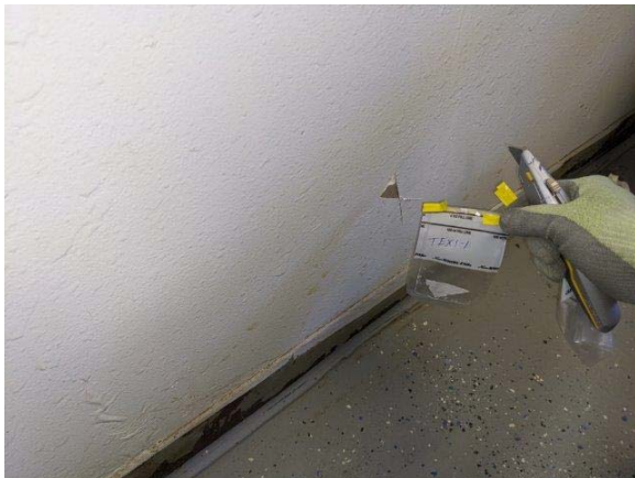
Sample: TEX1-1 - Drywall surface texture (orange peel) Result: Non-Detect
