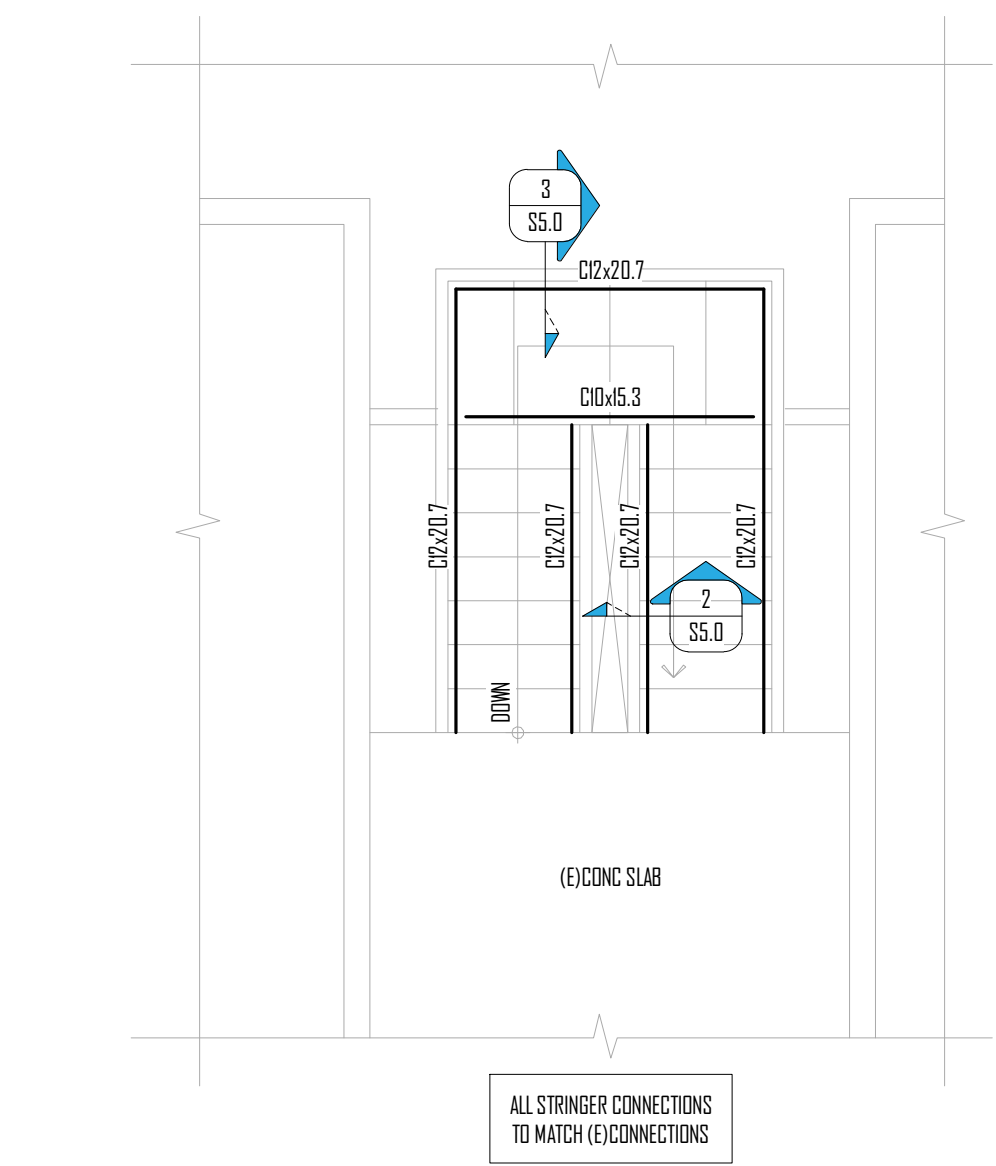
6 STAIR 20 SECOND LEVEL STAIR PLAN 1/4" = 1'-0"
